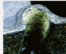
The edge of an A360 aluminum alloy conduit box after an industry-standard salt spray test.
