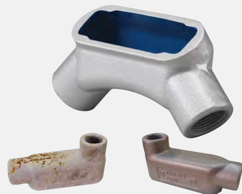
After a 500-hour 5% salt fog test, the standard galvanized iron conduit body has severe salt adhesion and significant rusting.
