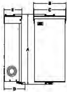
NEMA Type 3R Outdoor enclosure
