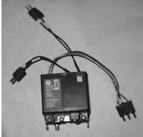
Network Interlock Device (NI)
