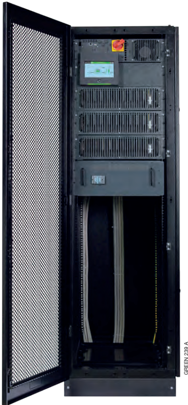
Example of integration (3x25 kW). Only 15 U of rack space occupied: space-saving design leaving free space for other rack-mounted devices. One empty slot in the MODULYS RM GP sub-rack remains available for power upgrade or redundancy.
