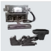
3rd rail Current Collector Device
