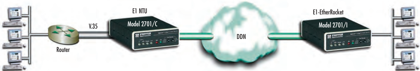
Models 2701 & 2701RC application: E1 network termination on X.21 or V.35 for data
