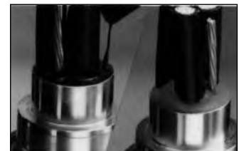
4. Pot cable (using liquid or putty)
