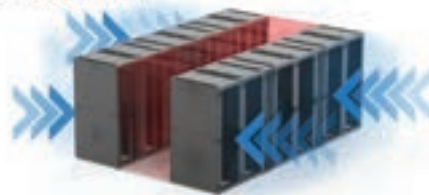
Hot aisle containment
