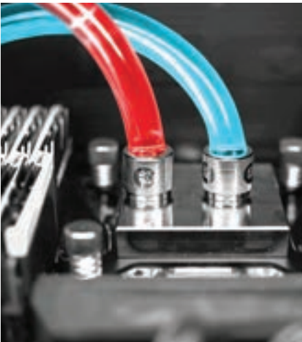
Cold Plate (Chip Level Cooling)
