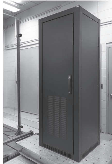
Enclosure mounted on shaker table
