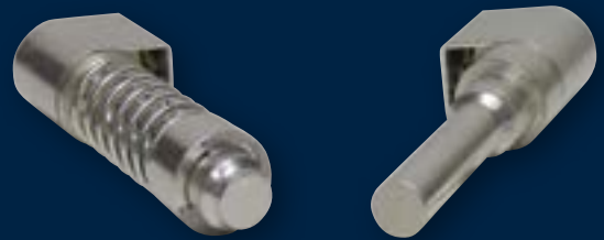
Silver-Nickel Contact Tip (85% Ag and 15% Ni)
