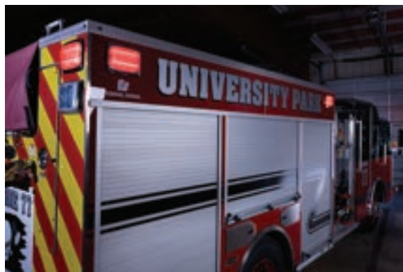
FireRay LED 9x7 (FR9C1-R) mounted on side and rear of fire engine
