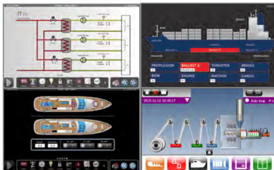
Screen built in Panel builder 800
