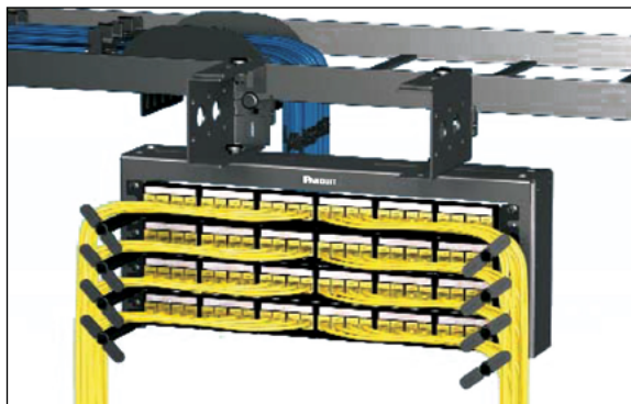
Mounted to side rail below ladder deck
