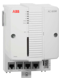
AC 800M process PLC, PM858
