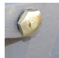
Grease pressure reliefs act to battle overgreasing
