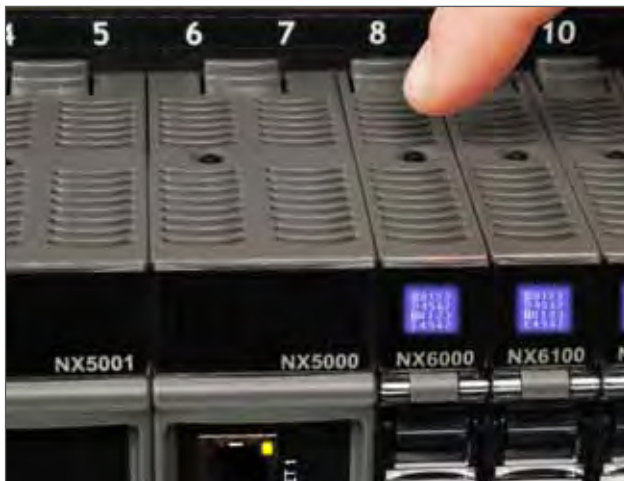
One-touch diagnosis with vivid alphanumeric LCD display affords instant troubleshooting at your fingertips.
