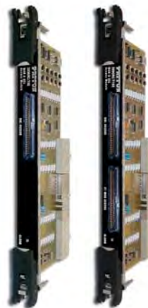
Rear transition modules with flexible interface capabilities
