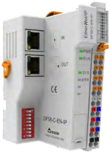
EtherNet/IP, 2 RJ45, extensible 32 modules, 24VDC
